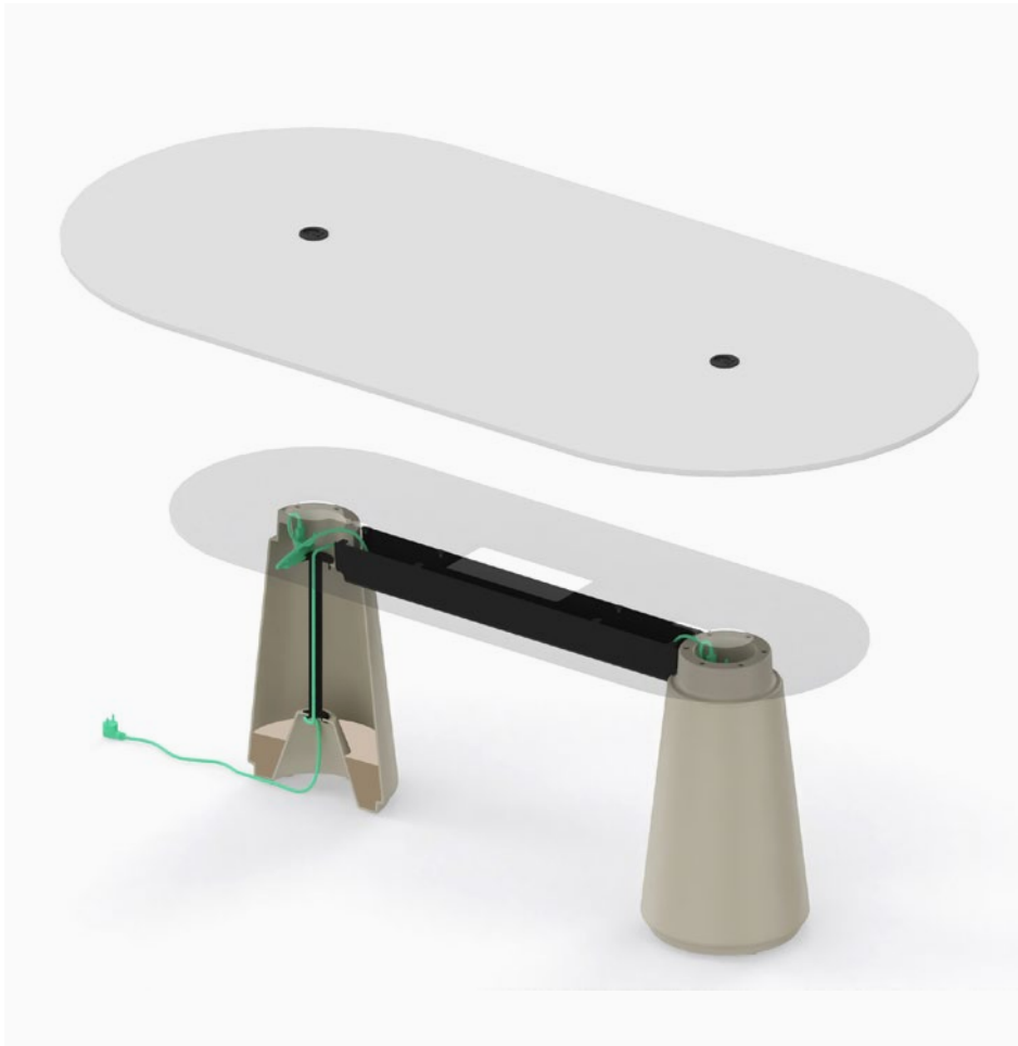
Integrated electrical management consisting of an electrified column and an electrification trunking connecting the two columns. One of the two columns is electrified with an inner tube made of steel with a diameter of 40 mm and bolted to the bottom of the column. The electrification tray is made of folded sheet steel with a thickness of 3 mm.
